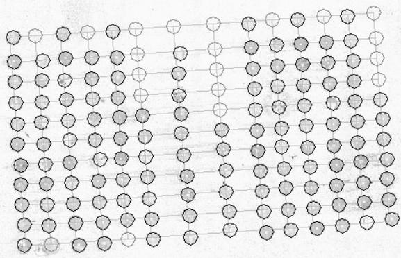
**Figure 2. Registered image map with super-imposed grid. Dark circles shows detected tissue discs, light circles show place holder grid positions.**
